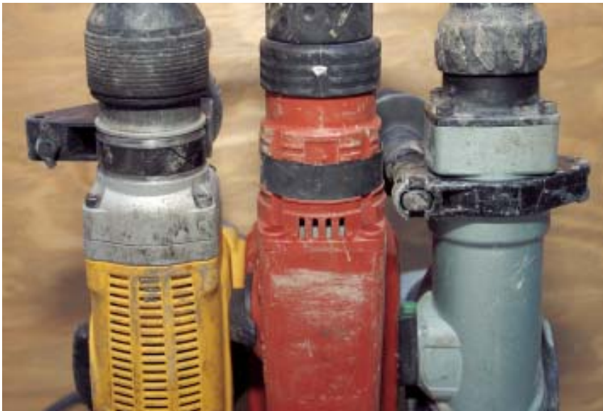
Figure 1. Most side handles attach to the tool with a metal band. The band on the DeWalt (left) is narrow and is tied to a very long handle, so there's a lot of flex in the connection. The band on the Hilti (center) is slightly wider; it's attached to a shorter handle, so there's much less give. Somewhat heavier than the other two bands, the thick steel clamp on the Hitachi (right) provides the most solid connection of all.
