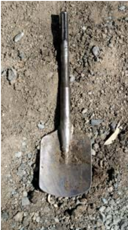
Figure 3. A clay spade (left) is indispensable for loosening packed soil, especially in cramped quarters. Here, a carpenter uses a combination hammer with a clay spade to help dig a trench (right).
