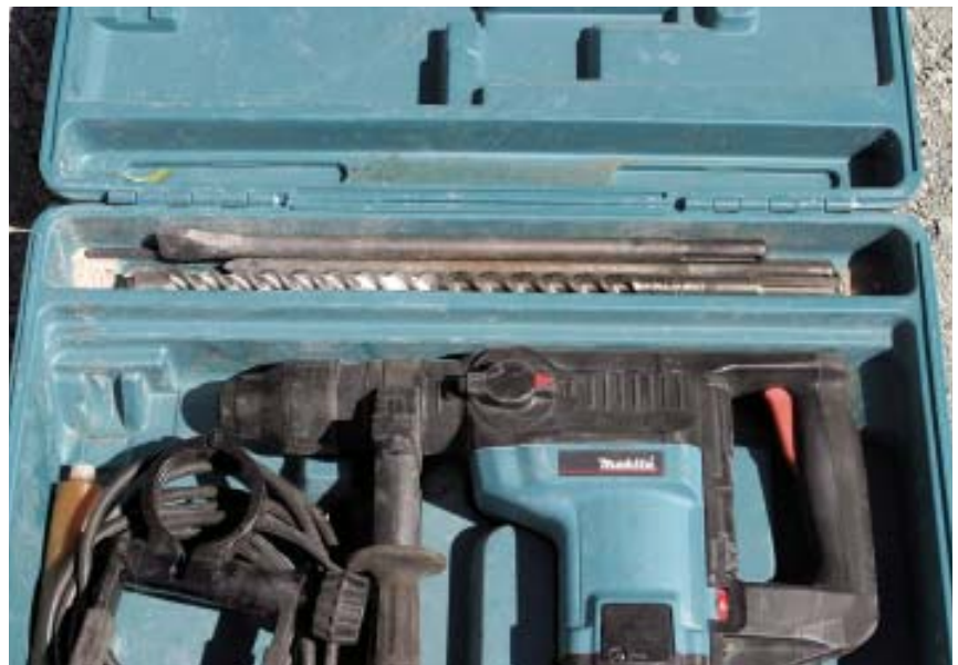
Figure 2. Like most of the cases that come with these tools, Hilti's (top) has room for multiple bits, chisels, and a clay spade. The Makita case (above) is cramped, with room for only a few small bits.
