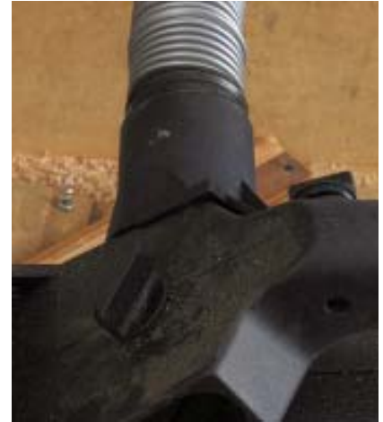
Figure 6. Both the Bosch (left) and the Festool (below) have adjustable two-side dust ports; the Porter-Cable has no dust collection.
