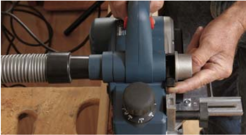
Figure 6. Both the Bosch (left) and the Festool (below) have adjustable two-side dust ports; the Porter-Cable has no dust collection.
