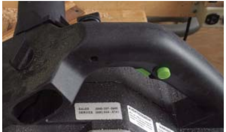
Figure 2. The safety lockout button on the Bosch planer (left) is in front of the trigger, so you have to either use two hands to start the tool or switch hand positions after starting it. The Festool's safety switch is near the trigger (right). The Porter-Cable has no safety lockout.
