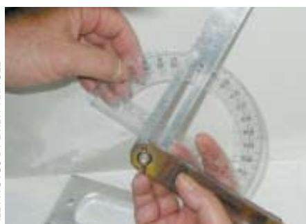
The inconvenience of using a bevel and protractor on an elaborate trim job compelled the author to come up with a better method to measure inside and outside corners. The ProSite Protractor not only measures the angle, it gives the correct miter setting for the saw.
