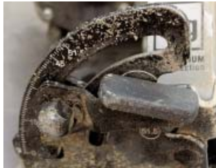
The bevel gauge is clearly marked and the blade tilts to 51.5 degrees.
