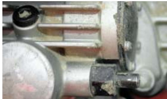
Ridgid's R3210 is a true worm-drive: Its hex fitting is the oil plug. The black button at the center of this photo is a spindle lock for changing the blade.
