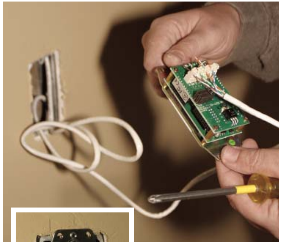
Figure 8. Four twisted pairs of Cat-5e cable clip into the back of a wall-mounted control device (above). Once installed, the device will control the speaker volume in the room and access an audio system that is installed elsewhere in the house (left).
