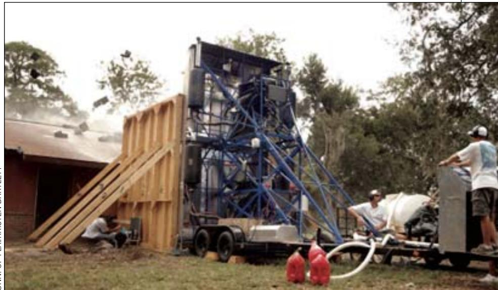
Shingles and tar paper fly off of the roof of a vacant home in central Florida as a custom-built wind machine pounds it with hurricane-force winds. Part of a University of Florida-led hurricane research project, the experiment was one of several aimed at learning more about how hurricanes damage homes that were built before Florida adopted its first statewide building code in 1994.
