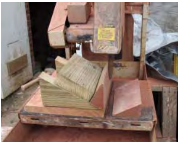
Figure 4. The author used jigs mounted on the sliding table of his brick saw for the angled cuts needed for the wing walls (top). For the mitered course topping the wing wall, he screwed an angled 2x2 to a plywood scrap (center). A second jig made with 2-by triangles held the bricks for the angled rip cuts needed for the wing wall's rowlock border (bottom).
