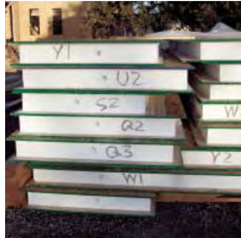
Figure 1. The most common type of structural insulated panel is produced by sandwiching EPS foam between two sheets of OSB. The face material can also be plywood, steel, or fiber-cement, and the core can be polyurethane.
