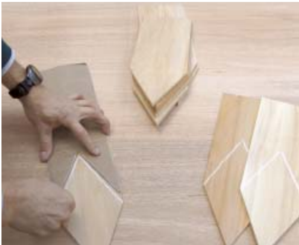
Figure 1. Pointed and reverse-point shingles (top) are cut on the same angle, using shingles of the same width for a balanced look. To make sure he keeps nails out of the exposure area, the author marks the pointed shingles with a cardboard template (above).
