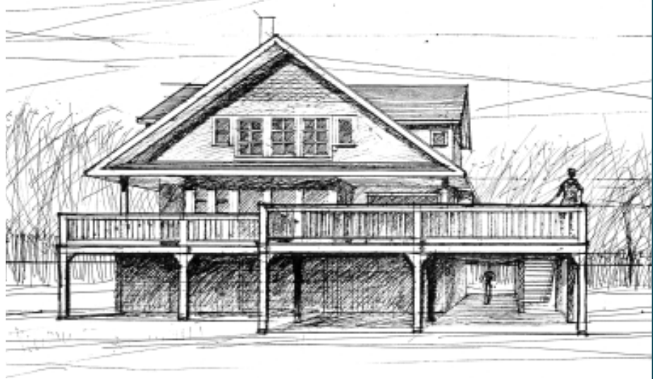
FIGURE 4. TULLY DESIGN. The low, wide eaves of the Tully design — reminiscent of the Fortier house — work with the extended porch to disguise the true height of the building.
