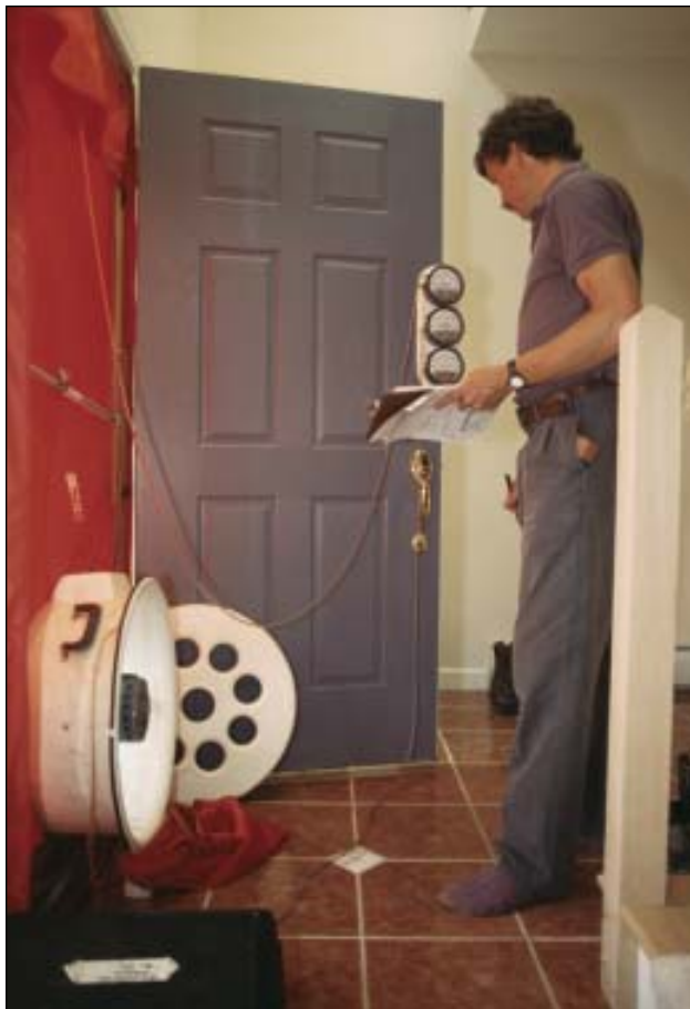
FIGURE 1. A blower door consists of a powerful fan that is temporarily sealed into an exterior doorway of a house. The fan blows air out of the house to create a slight pressure difference between inside and outside. House airtightness is determined by the amount of air-flow that it takes to maintain a 50 Pascal depressurization of the house. The tighter the house, the less air that's needed to exhaust in order to maintain the pressure.
