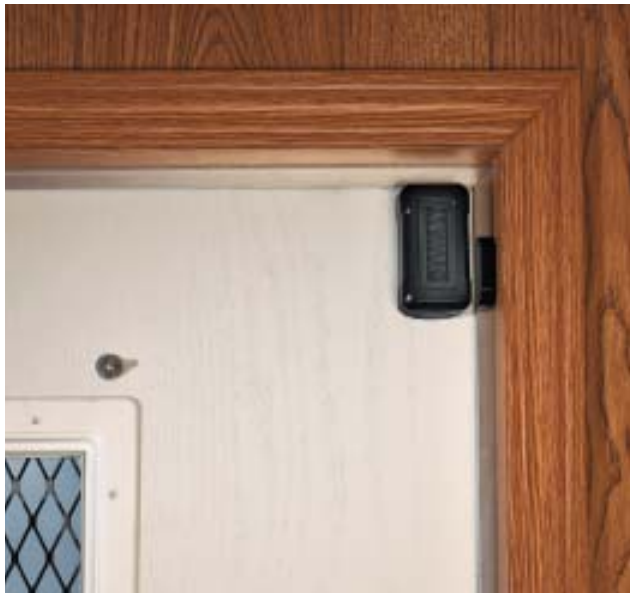
Figure 5. This wireless door/window contact is being used to protect the door of a job-site trailer. Wireless motion detectors similar to the ones used in home-security systems are also available for use with the Sitelock.
