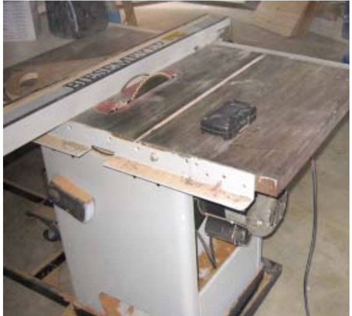
Figure 4. Container sensors are typically installed on job boxes and stationary equipment. This sensor is magnetically attached to the table saw; the alarm will go off if someone removes it or tries to move the saw.
