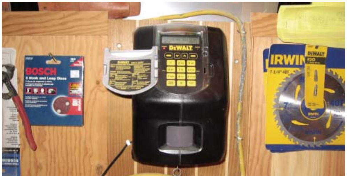
Figure 1. The base unit can be used alone to protect the area where it's installed or in conjunction with wireless sensors at various locations around the site. If a sensor is tripped, the base unit uses a built-in cellphone or land-line backup to send an alarm signal to the monitoring service.
