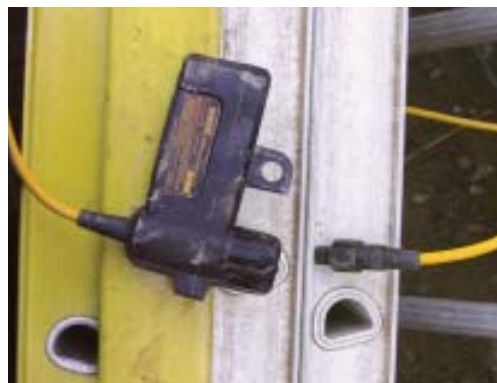
Figure 3. A cable sensor works like an electronic bike lock (above). If someone cuts or unplugs the cable while the system is armed, a signal travels to the base unit and the alarm goes off. The loose end of the cable (right) plugs into the locking device and can be secured with a padlock for added security (far right).
