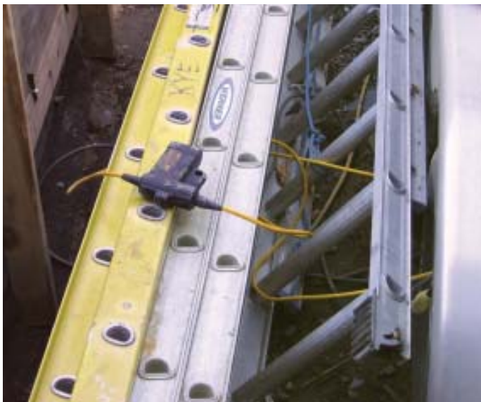
Figure 3. A cable sensor works like an electronic bike lock (above). If someone cuts or unplugs the cable while the system is armed, a signal travels to the base unit and the alarm goes off. The loose end of the cable (right) plugs into the locking device and can be secured with a padlock for added security (far right).
