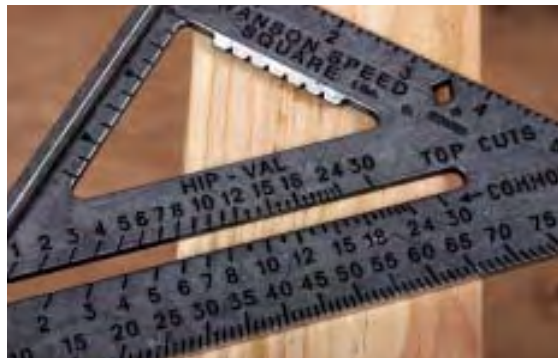
Figure 3. The rafters for a tray ceiling have plumb cuts on both ends. To use a Speed Square to lay out the 8/12 plumb cut on the end of a common, set the pivot point against the edge of the stock and align the number 8 on the "COMMON" scale with the edge of the stock (top). Use the same method to lay out the 8/12 plumb cut on the hip, but index off the "HIP-VAL" scale (above).
