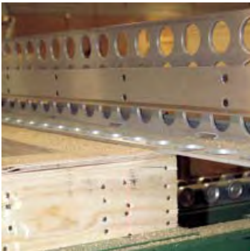
Figure 7. Before the panel is sheathed, it's pushed into shape on the squaring table, which is checked daily for accuracy. Pneumatic rams and a pawl on one end squeeze the panel while the sheathing is fastened (above left). In more automated shops, the sheathing nailer, which weighs 100 pounds, might be robotically positioned, but on this line the task is done manually by two people (above) with the help of a laser (left).
