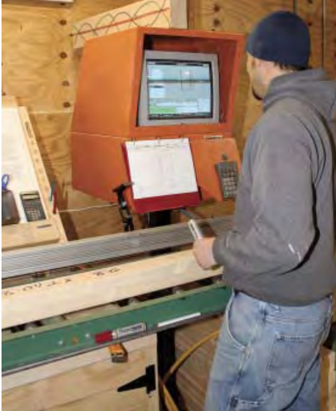
Figure 3. Shop drawings of individual wall panels are kept in a binder at the plate marker, the first machine on the panel assembly line (above). After the operator enters the panel number on the computer control, the machine uses a robotic stop (above right) for cutting the plates and marking the stud locations (right). The operator then tells the computer that the panel is complete, removes the shop drawing from the binder, and staples it to the plates. The machine won't allow the operator to mistakenly produce two of the same panels.
