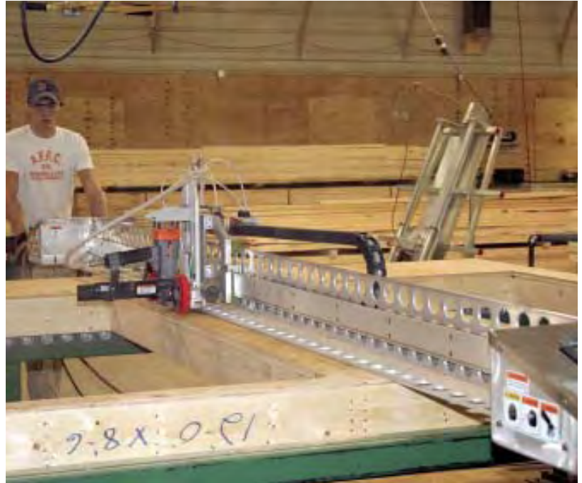
Figure 7. Before the panel is sheathed, it's pushed into shape on the squaring table, which is checked daily for accuracy. Pneumatic rams and a pawl on one end squeeze the panel while the sheathing is fastened (above left). In more automated shops, the sheathing nailer, which weighs 100 pounds, might be robotically positioned, but on this line the task is done manually by two people (above) with the help of a laser (left).
