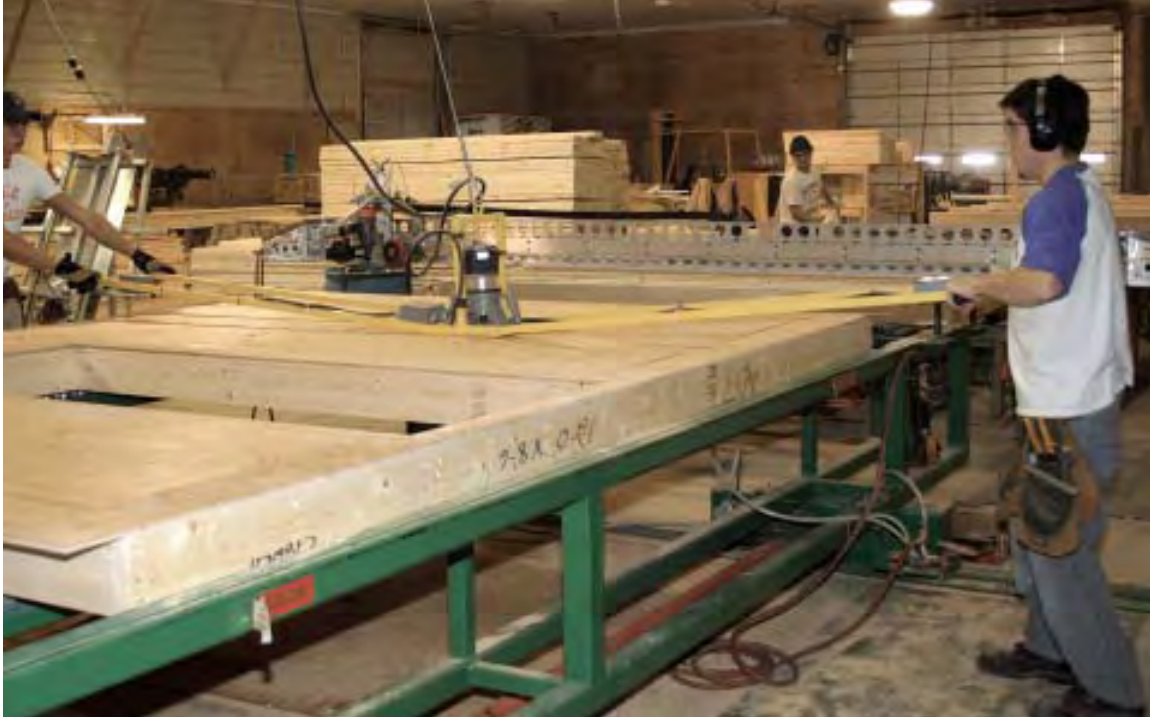
Figure 6. Window and door openings are cut with a 3 1 / 4 -hp router mounted on a steel sled. Suspended from a cable, it retracts out of the way when not in use and can cut out a door or window in about a minute.
