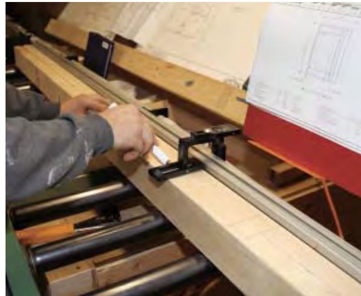
Figure 3. Shop drawings of individual wall panels are kept in a binder at the plate marker, the first machine on the panel assembly line (above). After the operator enters the panel number on the computer control, the machine uses a robotic stop (above right) for cutting the plates and marking the stud locations (right). The operator then tells the computer that the panel is complete, removes the shop drawing from the binder, and staples it to the plates. The machine won't allow the operator to mistakenly produce two of the same panels.
