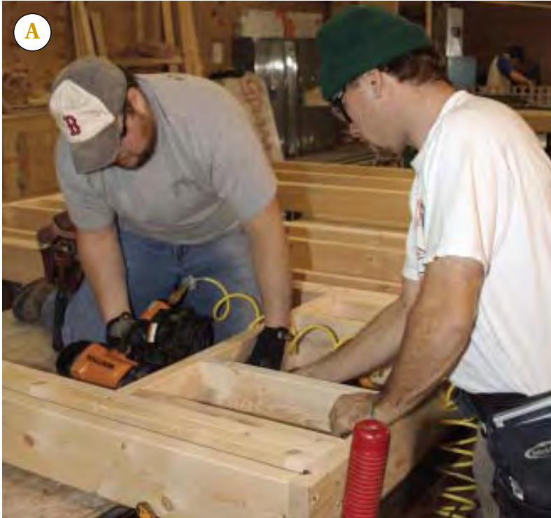
Figure 5. At the framing table, the subcomponents are the first pieces fastened to the plates, along with any cripple studs (A). Steel fingers (painted yellow) ensure accurate 16-inch o.c. spacing and can pivot to lay flat when they interfere with the placement of a double stud, tee, or header (B). Once the remaining studs are placed, the whole panel is held together with pneumatic rams while it's nailed off with special weight-assisted two-gang framing nailers (C). Before the panel moves on, any twisted studs are pried into place with a tweaker (D) before being nailed with a pneumatic nailer; blind cavities are filled with insulation (E).
