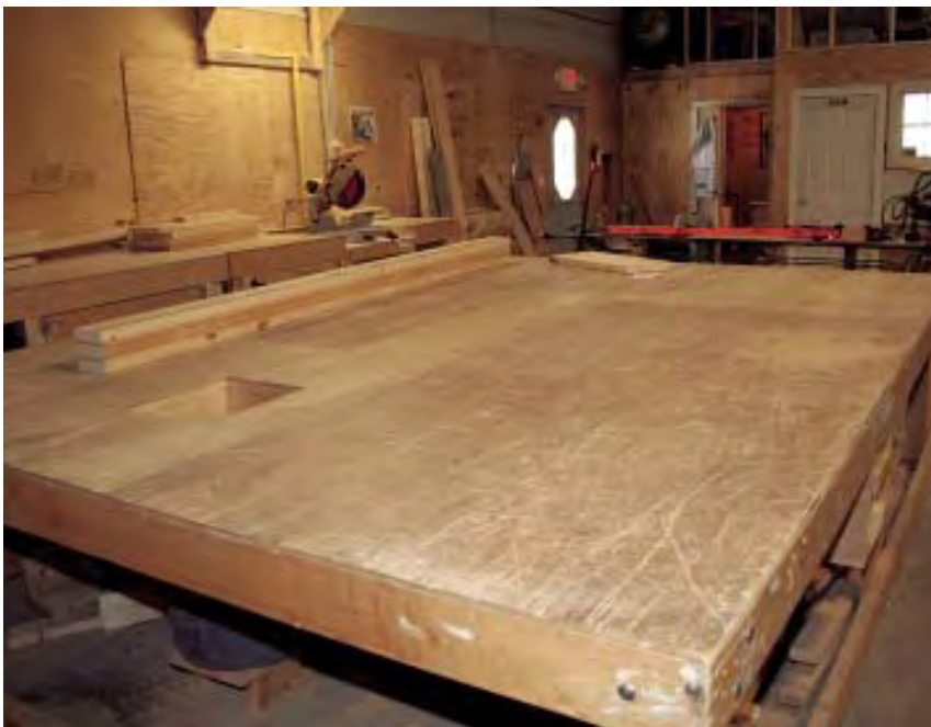
Figure 1. Before switching to a semiautomated assembly line, the author used a pair of assembly tables like this one to build his wall panels. The waist-high tables make framing easier on the back and can include layout marks and jigs to speed production. Once a wall panel is framed and sheathed, it's slid onto a rolling cart or forklift. The hole in the table is for scraps; a barrel sits underneath.
