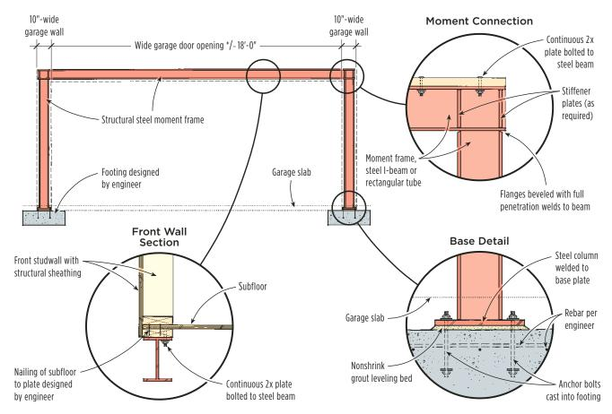
A moment frame can be used to provide shear strength for narrow-walled structures when standard framing solutions are inadequate. In all cases, beam and column sizes and connection details need to be designed by a structural engineer.
