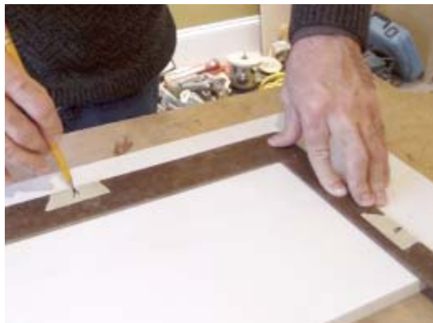
Figure 1. The key to the Up System is an accurate measurement of the stair's rise and run. Here, the author lays a framing square onto a tread and transfers these dimensions to the square (above). Next, he places the framing square on a piece of paper or a scrap of plywood and draws a full-scale right triangle, with the base of the triangle equal to the stair's run and the height of the triangle equal to the stair's rise (right).
