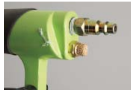
Figure 5. Several of the pinners have nonadjustable exhaust ports (left); the Nikle (above left) has a swiveling exhaust on the head. The author's favorite tools have a rear filtered exhaust (above), which completely dampens the blast of air.
