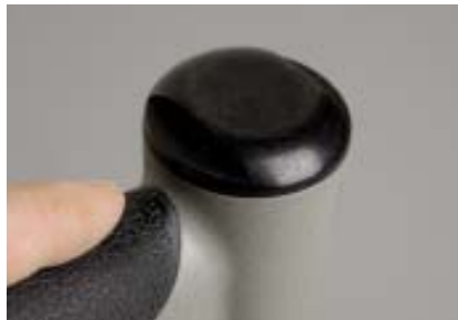
Figure 5. Several of the pinners have nonadjustable exhaust ports (left); the Nikle (above left) has a swiveling exhaust on the head. The author's favorite tools have a rear filtered exhaust (above), which completely dampens the blast of air.
