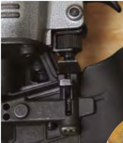
Figure 4. On most roofing nailers, depth-of-drive is adjusted by turning a thumb-wheel on the nose or near the trigger, as on the Senco gun (above). The depth-of-drive on the Bostitch (right) is especially easy to adjust because the mechanism is controlled by a large knob on the nose.
