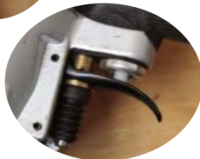
Figure 3. A well-designed trigger can make a difference. The trigger on the Paslode tool (top left) is especially comfortable because it's contoured and long enough to fit two fingers. Ridgid's trigger (left) curves down and has a soft rubber pad. The bare-bones trigger on the Spotnails gun (below) is identical to the trigger on the Hitachi tools.
