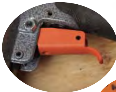
Figure 3. A well-designed trigger can make a difference. The trigger on the Paslode tool (top left) is especially comfortable because it's contoured and long enough to fit two fingers. Ridgid's trigger (left) curves down and has a soft rubber pad. The bare-bones trigger on the Spotnails gun (below) is identical to the trigger on the Hitachi tools.
