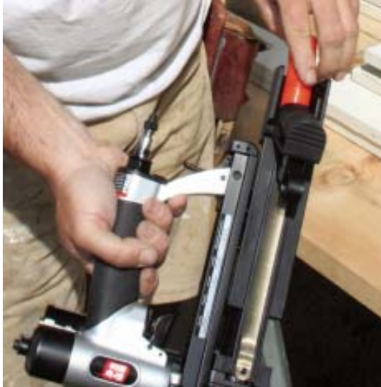
Figure 4. The Grip-Rite's cap magazine is mounted on the bottom of the tool — rather than on the side, as with the other guns. This arrangement makes the Grip-Rite very compact. To load the caps, the user retracts the cap pusher, which opens the magazine door; strings of 110 caps go in the end (above). The author found this cap-feed system unreliable. Staples go in a separate magazine under the handle (right).
