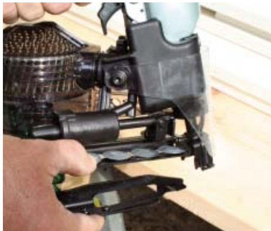
Figure 5. Loading the Hitachi takes some effort: First you have to open two doors to load the nails and engage them on the feed pawls (far left). Then you open the cap magazine and get the caps started on the feed mechanism (left). It took the author several attempts to master the process.
