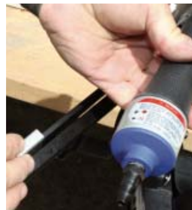
Figure 6. The Spotnails' circular magazine accepts 200 caps. Once they're loaded, the caps advance manually while the user holds up the "picker's" red handle (left). Staples can be placed on the magazine rail after the pusher is locked in the retracted position (right).
