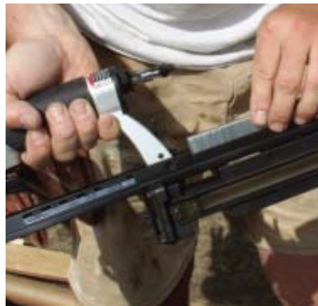
Figure 4. The Grip-Rite's cap magazine is mounted on the bottom of the tool — rather than on the side, as with the other guns. This arrangement makes the Grip-Rite very compact. To load the caps, the user retracts the cap pusher, which opens the magazine door; strings of 110 caps go in the end (above). The author found this cap-feed system unreliable. Staples go in a separate magazine under the handle (right).
