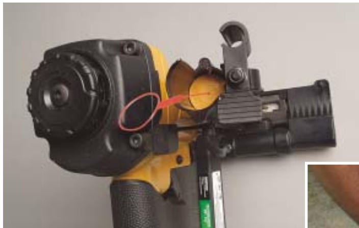
Figure 3. Bostitch's vertical cap magazine, which is made from sturdy reinforced plastic, is the easiest to load. With the pusher pulled to the top and rotated out of the way, strings of caps are dropped in (left). Once the pusher is back in place, the plastic leader is pulled out. Stacked caps like Bostitch's (below) fit better in a toolbelt and are less vulnerable to damage than coiled caps.
