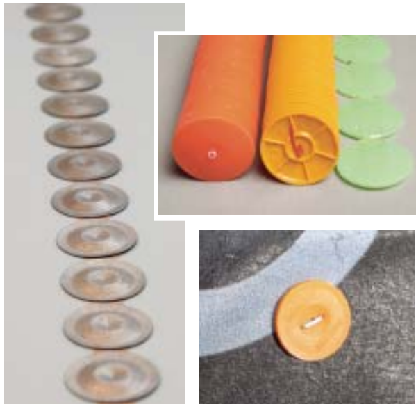
Figure 2. The author likes stacks of caps better than coils. Coils tend to unroll and become distorted, making loading difficult. Hitachi offers coils of caps in both metal and plastic; its metal cap is shown here (left). The other tools use plastic caps (top right, from left: Grip-Rite, Bostitch, Spotnails). Caps measure about 1 inch in diameter. A properly driven cap sits tight to the roof without distortion (above right).
