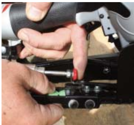
Figure 6. The Spotnails' circular magazine accepts 200 caps. Once they're loaded, the caps advance manually while the user holds up the "picker's" red handle (left). Staples can be placed on the magazine rail after the pusher is locked in the retracted position (right).
