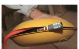
The author stows an air hose by wrapping it around the perimeter of the largest Cordpro, the CP-XL (left). The sides of the Cordpro spring open, allowing a hose or cord to slip inside (right).
