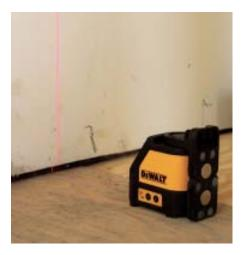
This laser is about 6 inches off the wall with the plumb beam on. The vertical line is visible all the way up the wall and about 2 feet out onto the ceiling above.
