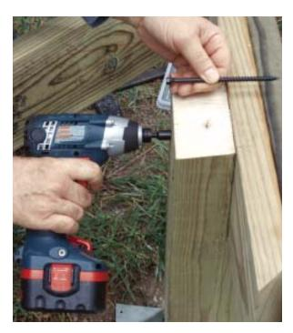
At only  $6^{1/2}$  inches wide, the Impactor fits in spaces too small for conventional cordless driver/drills. And with 1,150 inch-pounds of available torque, it can drive 5-inch fasteners into southern yellow pine without predrilling.
