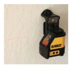
Two on/off buttons control the DW087, one for level lines and the other for plumb. In this photo, the horizontal beam is on and the magnets are holding the unit to the wall bracket, which hangs from a nail in the wall.
