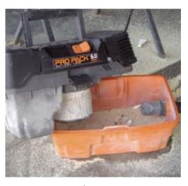
The 4<sup>1</sup>/<sub>2</sub>-gallon-capacity vacuum captures small particles with a pleated paper filter. The maker recommends removing the filter for wet pickup.
