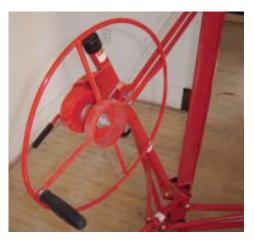
The lift's winch is a little choppy, and the hand-wheel that controls it is noticeably off-center. These problems don't affect operation greatly, though, and the most important control—the lift brake—works just fine.
