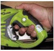
The Worx recip saw's grip pivots over a 60-degree range and can be locked in various positions; here it's shown in the straight position (left) and rotated all the way down (right).
