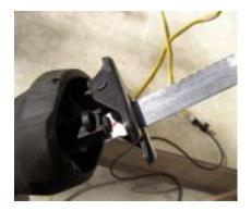
The blade clamp is tucked into the nose of the saw, so it's harder to get to than the clamps on other models.
