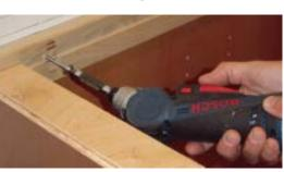
The PS10's 10.8-volt lithium-ion battery pack provides a surprisingly long runtime for smaller fasteners. However, the author's self-drilling cabinet screws proved too much for the tool - despite the manufacturer's claim that one charge delivers enough power to drive 100 3-inch screws.
