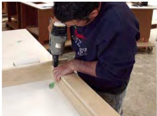
Figure 9. With a completed jamb assembly on the bench, the author prepares to attach the side casings. Hot-melt holds the biscuits in the slots (above) and the casing against the side jambs' exterior face, automatically governing the finish reveal (above right). Finish nails complete the assembly (right).
