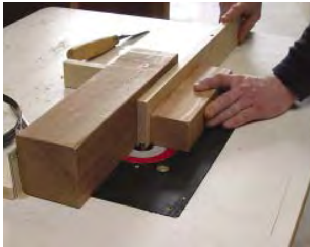
Figure 4. A routed groove in the extension jamb head will receive the \frac{3}{8} -inch-wide parting bead, making a strong, self-aligning connection between the two parts.
