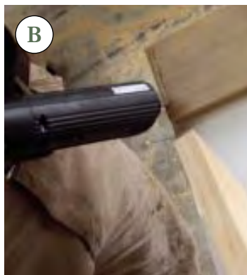
Figure 5. Three-piece extension jamb sets are laid out on the table for assembly, six at a time (A). Polyurethane hot-melt adhesive provides a strong 30-second bond between parts, allowing accurate and secure alignment (B). Trim-head screws add strength to the glued joint (C). Completed jamb sets are stacked to one side, awaiting the next assembly step (D).
