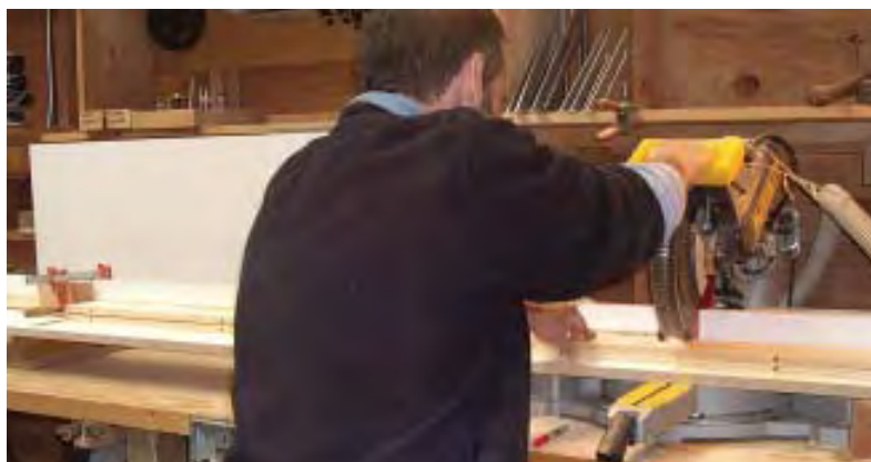
Figure 3. Here, the author's layout stick is clamped to an auxiliary fence on his chop saw (top). Colored lettering matches the layout stick to the white offset stick, which provides the lengthening dimensions for reveals, stock thickness, and overhangs (center). With a stop block clamped at the appropriate layout mark, the author can cut side extension jambs two at a time (above).
