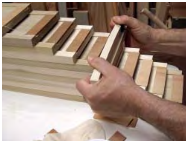
Figure 10. Fillets hide the gaps at head casing and apron ends. The author uses a block of wood to press the fillets down flush in a bead of hot-melt glue.
