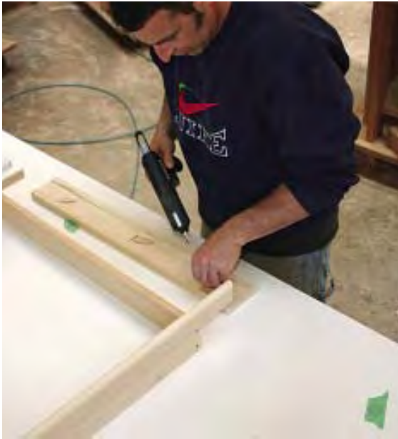
Figure 9. With a completed jamb assembly on the bench, the author prepares to attach the side casings. Hot-melt holds the biscuits in the slots (above) and the casing against the side jambs' exterior face, automatically governing the finish reveal (above right). Finish nails complete the assembly (right).
