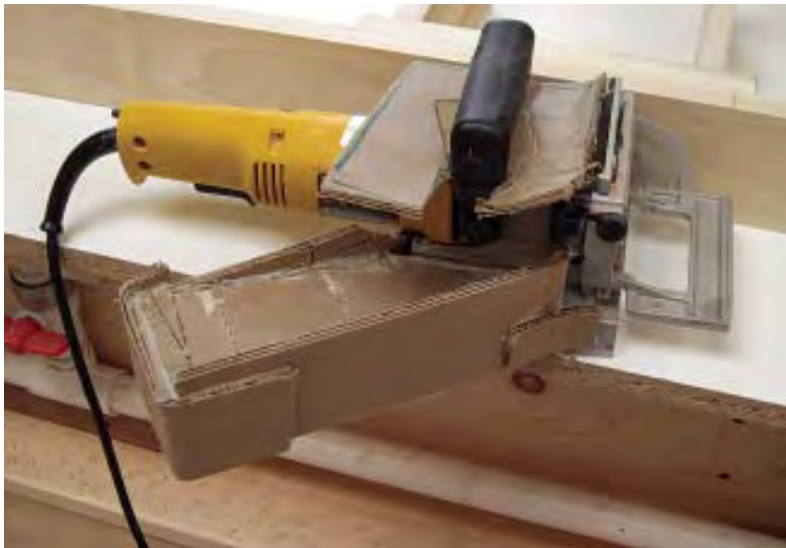
Figure 8. The author uses wood joining biscuits to govern his casing reveals. The backing fence against which the stock is being pressed is hot-melt-glued to the workbench and has center marks along its top edge to guide the biscuit joiner. Stock stacked five deep in front of the fence receives a series of slots in a single, repetitive operation (top). Cardboard hot-melt-glued to the biscuit joiner deflects chip exhaust onto the floor (above).
