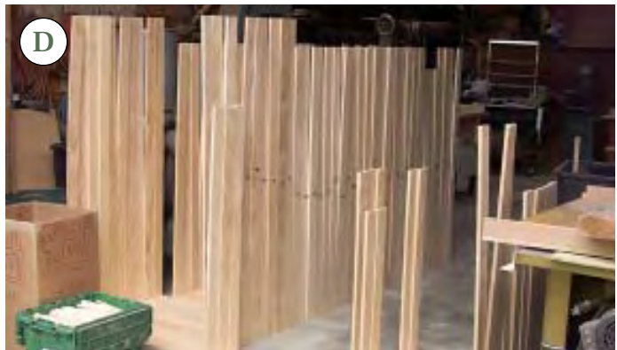
Figure 5. Three-piece extension jamb sets are laid out on the table for assembly, six at a time (A). Polyurethane hot-melt adhesive provides a strong 30-second bond between parts, allowing accurate and secure alignment (B). Trim-head screws add strength to the glued joint (C). Completed jamb sets are stacked to one side, awaiting the next assembly step (D).
