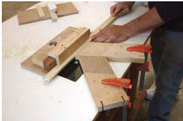
Figure 6. The author's shop-made router fence has a built-in dust port to reduce chip buildup (top). A hold-down is screwed to the fence to control the stock feed, while front and rear stops on the end-milling sled help prevent grain tear-out (center). After rounding all the ends, the author sends the long edges through the router table. This sequence wipes out any minor tear-out that may have occurred during end-milling. Dual feather boards ensure absolute stability (above).
