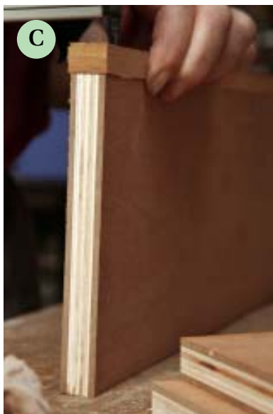
Figure 1. To strengthen the bookcase so it wouldn't sag, the author cut dados for the shelves (A). Before applying solid wood banding to the shelf edges, he ran them over a Collins Ply Prep bit (B), which helps achieve a tight glue line (C). The finished side on the strike side had to be beveled (D) to clear the jamb.
