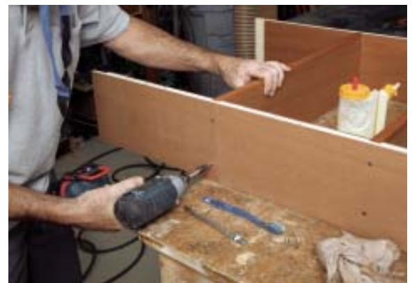
Figure 2. After prefinishing the pieces (above), the author assembled the case with glue (top right) and screws (right).
