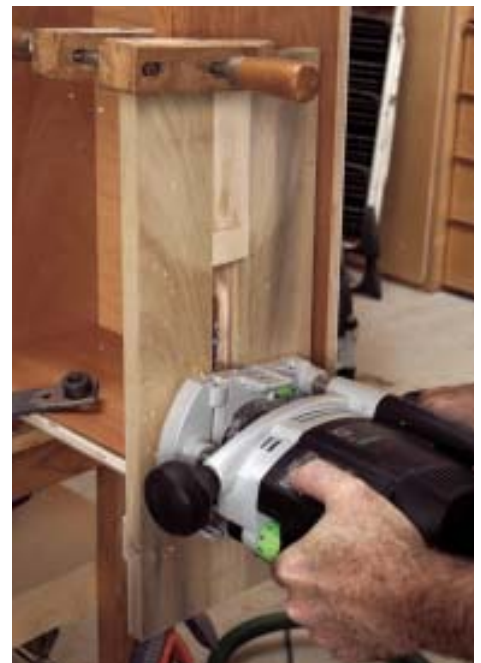
Figure 3. This Rixson pivot hinge set (top left) has a 500-pound capacity. The author made router templates (left) to guarantee that the mortises in the case and jambs would be accurate (above).
