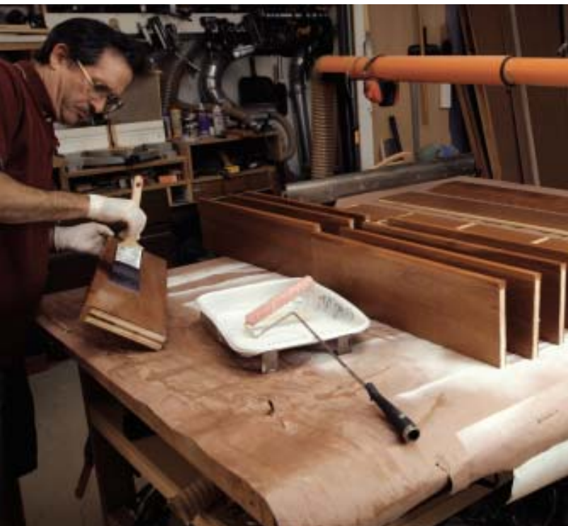
Figure 2. After prefinishing the pieces (above), the author assembled the case with glue (top right) and screws (right).
