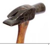
The cross-peen head on this 1867 combination hammer — like that on a modern cabinet-maker's hammer — was used for driving brads or tacks.
