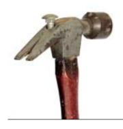
This nifty hammer of unknown date and manufacture may be an inventor's prototype. It features an interchangeable face secured with an Allen bolt, presumably so the waffle-faced framing head could be exchanged for a lighter, smooth face for finish work. The carriage bolt in the threaded hole above the claws allowed the carpenter to adjust the amount of nail-pulling leverage required without having to hunt around for the right-size block.
