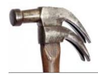
Designed to let the user switch from the lower to the upper set of claws partway through pulling a nail, the four-clawed Crusader hammer minimized bending — a useful feature in an age when thrifty carpenters routinely straightened and reused salvaged nails.
