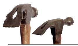
Who says a claw hammer has to have two (or more) claws? These early 20th-century mono-claw hammers look like they'd still be thoroughly useful today. Both feature an adze- or chisel-like blade with a central nail-pulling slot; the model at far left also has additional notches in the sides for pulling tacks or other small fasteners.
