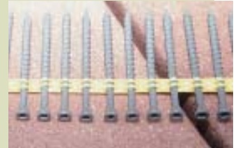
Figure 8. The decking is fastened with trim-head screws, which are buried slightly below the surface of the composite decking. Each screw creates a small “mushroom” that is hammered flat to conceal the screw head.
