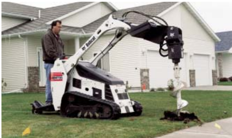
Figure 4. A walk-behind skid steer with an auger attachment makes quick work of footing holes, and can be rented on a daily basis.
