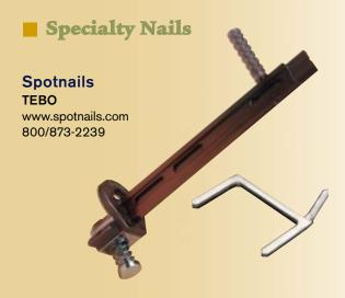
The TEBO is a three-pronged, stainless-steel connector that's driven with a special tool (\$300) and a mallet. When you drive it in, one prong enters the first deck board and the second enters the joist below — both at an angle that leaves the third prong parallel to the joist. With the first board secure, the next board is driven onto the third prong using a sledgehammer and a block. \*
