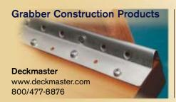
Available in a powder-coated version for most applications and a stainless-steel version for coastal use, the Deckmaster screws to the sides of the joists and the bottom of the decking. It comes in 22<sup>1</sup>/2-inch lengths that accommodate four nominal 6-inch deck boards. Installation requires either access from below, or working upside down from above.
