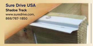
Shadoe Track is nailed or screwed to the tops of joists. Deck boards are attached with screws from below, and, again, access from below or lots of bending at the waist is called for. It comes in 8-foot lengths in galvanized, powder-coated, and stainless-steel versions.
