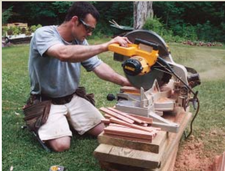
Figure 4. Cut from 9-inch-long scrap riser material, the wedges are beveled at 4 degrees, which is done by setting the saw to 2 degrees and flipping the stock end-for-end at each cut. The carpenter eyeballs the cuts so that the sharp ends of the wedges measure about \frac{3}{16} inch.
