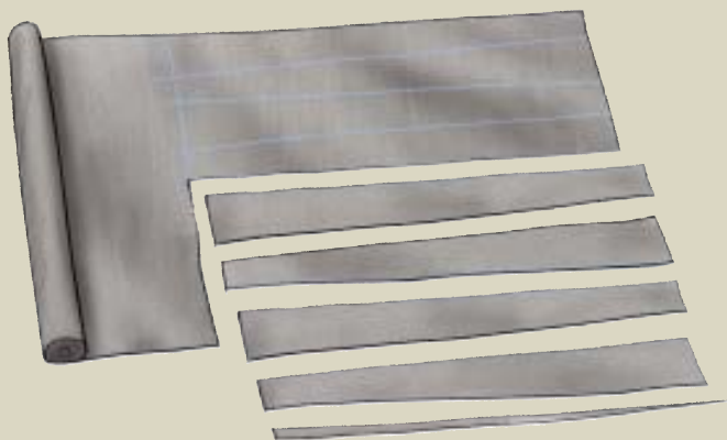
Figure 3. The string measurements are transferred to a layout, alternating wide and narrow ends across the width of an appropriate length of membrane. Cut lines are snapped with a chalkline.
