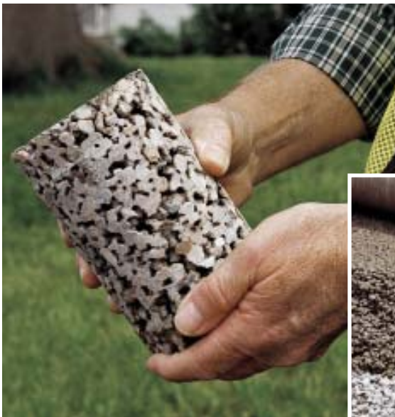
Figure 1. Made largely without fine aggregates, pervious concrete has a porous structure that allows up to 18 gallons of water per minute per square foot to flow through it — yet the material can have a compressive strength of more than 3,000 psi when fully cured.
