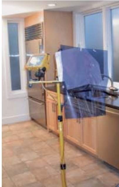
Figure 3. To match the 5,500 K color temperature of daylight, the author adds blue CTB conversion filters to his light sources (left). Then he experiments, strategically placing lights — such as this filtered and diffused pro light located in a hallway off the kitchen (right) — to achieve even, natural lighting.
