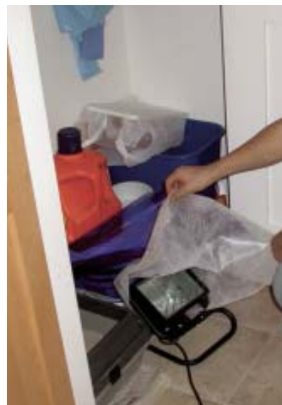
Figure 2. While professional light kits offer greater control and more features, basic work lights are an inexpensive and readily available light source for job-site photography. To soften shadows, bounce light off a reflective surface, such as a ceiling (left), or use heat-resistant spun-fiberglass diffusion material, which can be safely draped over hot work lights (bottom photos).
