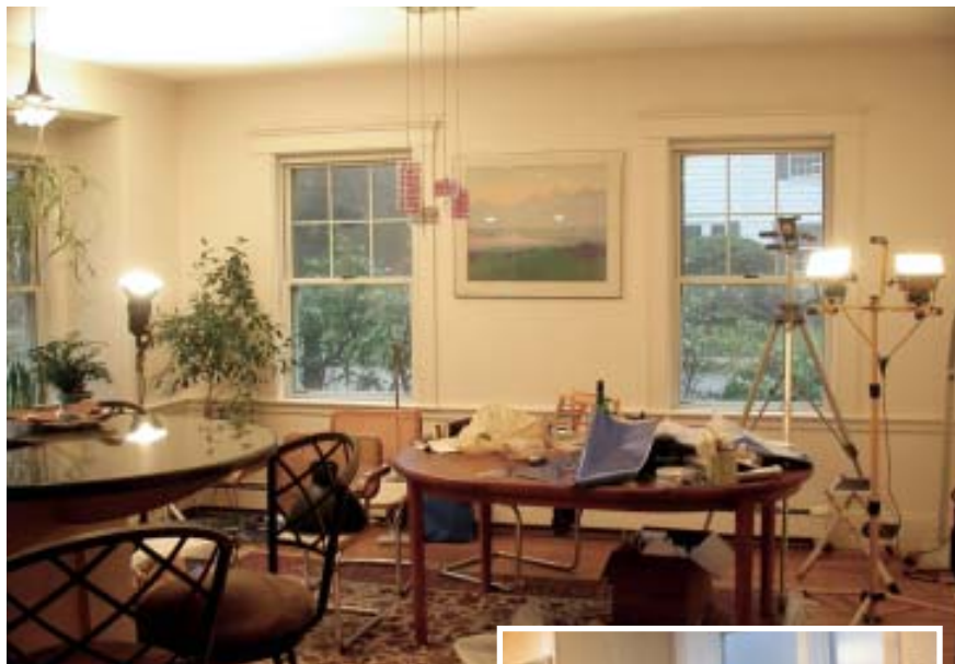
Figure 2. While professional light kits offer greater control and more features, basic work lights are an inexpensive and readily available light source for job-site photography. To soften shadows, bounce light off a reflective surface, such as a ceiling (left), or use heat-resistant spun-fiberglass diffusion material, which can be safely draped over hot work lights (bottom photos).
