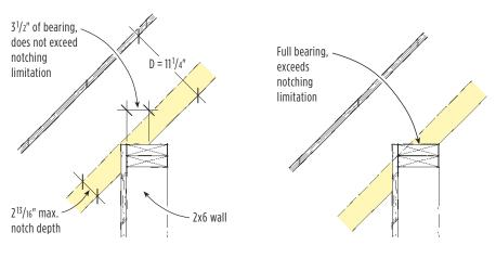
you still shouldn't overnotch. This is because larger knots are allowed in 2x10s and 2x12s than in 2x6s and 2x8s; overnotching a large rafter voids the grade stamp and may compromise the stock's structural integrity.
