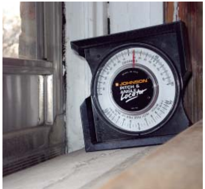
Figure 2. Marvin's insert replacement window can be made to virtually any sill angle; if the angle is 5 degrees or less, the insert will be constructed with a flat sill.
