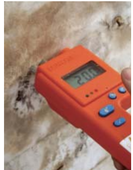
Figure 5. The author's crew used a hand-held moisture meter to measure the moisture levels in the OSB-covered SIP panels. Readings were highest around windows — which had been poorly flashed — and closer to grade, where water leaking in from above would have accumulated. Levels were lowest on the second floor under the eaves overhang.
