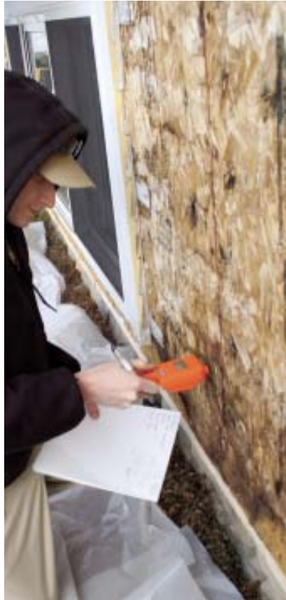
Figure 5. The author's crew used a hand-held moisture meter to measure the moisture levels in the OSB-covered SIP panels. Readings were highest around windows — which had been poorly flashed — and closer to grade, where water leaking in from above would have accumulated. Levels were lowest on the second floor under the eaves overhang.
