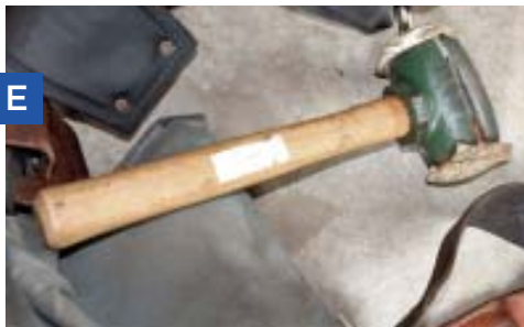
Figure 2. Specialized power tools from Mafell — a chain mortiser (A) and an oversized planer (B) and circular saw (C) — speed the prepping of timbers in the shop. On site, the crew uses a collection of large wood mallets (D) and smaller rawhide mallets (E) to nudge timbers into place, and large chisels (F) for fine-tuning joints. Most important of all, the company's boom truck (G) handles delivery and heavy lifting.
