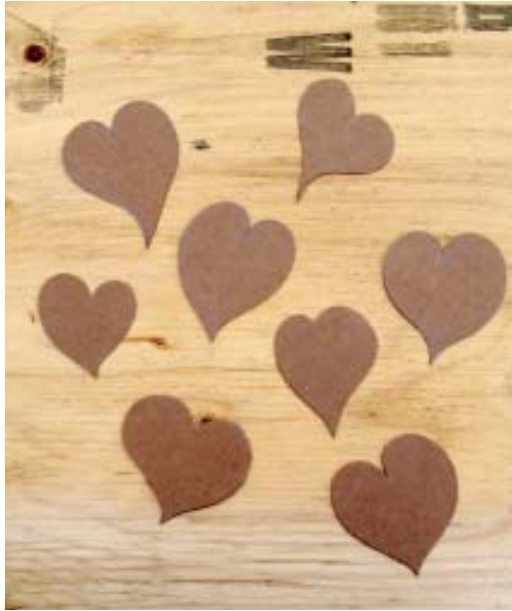
Figure 1. To simplify layout, the author prepares a series of leaf patterns. He draws them free-hand on heavy paper or cardboard and cuts them out to use as templates.
