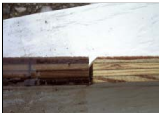
FIGURE 1. Saturated OSB (top) swells considerably, and does not shrink back to its original dimension when it dries out. Plywood soaked in the same way (above) does not swell to the same degree, remaining dimensionally stable.
