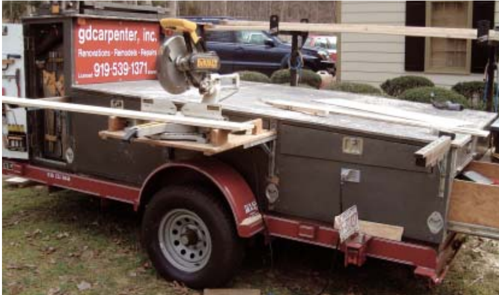
Figure 4. Removable shelf brackets hold a miter saw (left); folding shelf brackets serve as stock supports (below). Brackets attached to the rear of the trailer put a table saw at just the right height for the deck to be used as an outfeed table (bottom).
