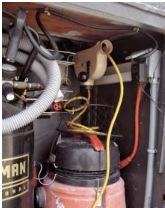
Figure 2. Inside the front compartment, an extension cord feeds to a GFCI outlet (left). From there, power is fed to a pair of outlets built into the sides of the trailer. Various storage spaces suit different tools: Delicate items have their own shallow niche (below), while larger ones reside in a series of drawers (bottom).
