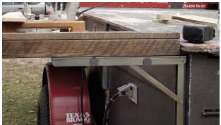
Figure 4. Removable shelf brackets hold a miter saw (left); folding shelf brackets serve as stock supports (below). Brackets attached to the rear of the trailer put a table saw at just the right height for the deck to be used as an outfeed table (bottom).
