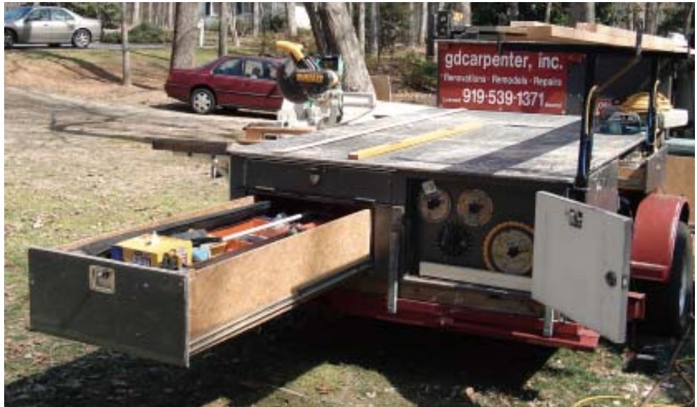
Figure 3. At the back of the trailer, a 6-foot drawer accommodates long tools — like a 6-foot level — and bins of electrical and plumbing supplies. It's the only drawer without a full extension.
