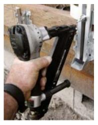
guns. Also, the GR150 tends to jam with the last few nails of the clip. (Actually, my other nailers do this, too.) To solve this problem, I load a new clip when there are still three or four nails left. I find that paper collated nails — though you have to keep them dry — work better than plastic collated. The plastic sometimes gets hung up inside the barrel, preventing the lead nail from protruding where I can see it.
