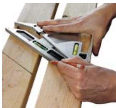
If all you do is build decks, this tool's price tag makes sense mostly if you're also a serious tool junkie, but it does have some applications for a deck builder. The Pivot Square functions as a speed square that can also accurately measure and transfer angles. It's got a place in stair work as well, as the integral level vials make it possible to measure pitch.
