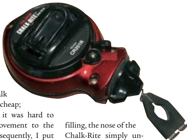
filling, the nose of the Chalk-Rite simply unscrews, and a barely noticeable detent has so far prevented the Chalk-Rite from opening unexpectedly. A thumb catch locks the reel, easing solo line snapping. The Chalk-Rite's gear-drive retrieves the line astonishingly quickly, which brings me to the best feature of this tool.
