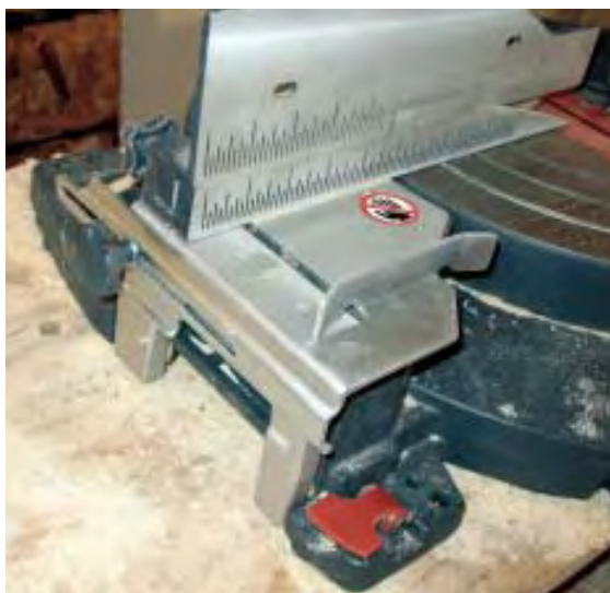
Figure 9. The adjustable crown stop supplied with the Bosch 4212L takes the guesswork out of positioning crown molding for upright cuts.
