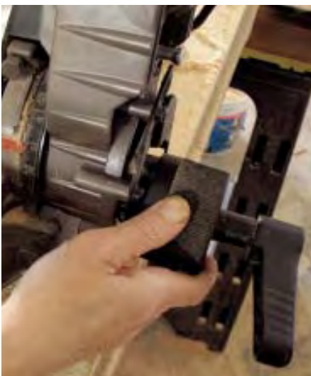
Figure 1. DeWalt's fast-acting cam-lock miter handle (above) proved superior to the screw-in knobs on the other machines. Among bevel controls, the front-mounted lever on the Bosch 4212L was the easiest to operate (above right), and the fine adjustment knob found on both Hitachi models made dialing in the exact setting particularly easy (right). The small black (right-mounted) switch on the DeWalt and the red (center-mounted) switch on the Bosch let users override the detent functions.
