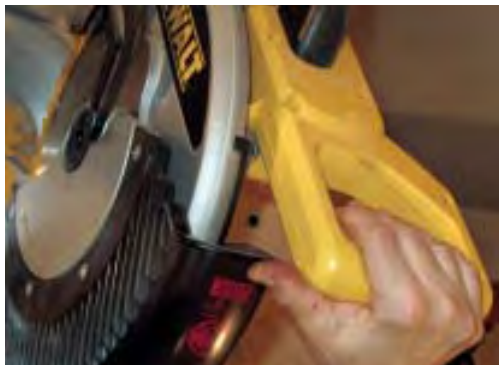
Figure 6. Sometimes it's necessary to raise the blade guard slightly to start a cut. The guards on the DeWalt (left) and Hitachi models were the easiest to elevate using only the trigger-hand thumb.
