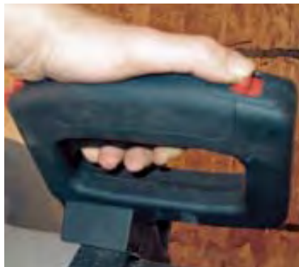
Figure 5. Four of the saws tested were outfitted with trigger-lock safety switches, the best and worst of which were on the Bosch models. Depressing the safety override (red button) along with the trigger on the Bosch 3912 (right) can be a stretch, especially for left-handers. The Bosch 4212L (far right) features a four-position adjustable grip that maximizes comfort.
