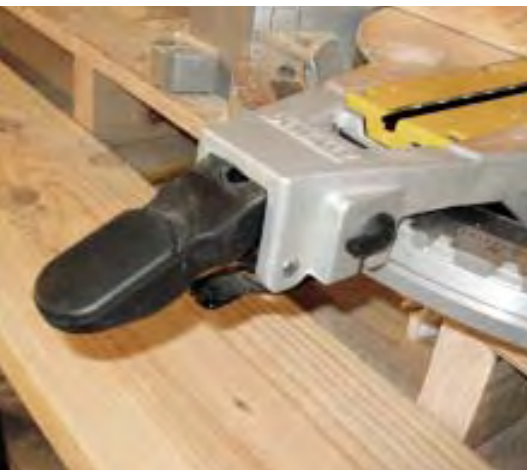
Figure 1. DeWalt's fast-acting cam-lock miter handle (above) proved superior to the screw-in knobs on the other machines. Among bevel controls, the front-mounted lever on the Bosch 4212L was the easiest to operate (above right), and the fine adjustment knob found on both Hitachi models made dialing in the exact setting particularly easy (right). The small black (right-mounted) switch on the DeWalt and the red (center-mounted) switch on the Bosch let users override the detent functions.
