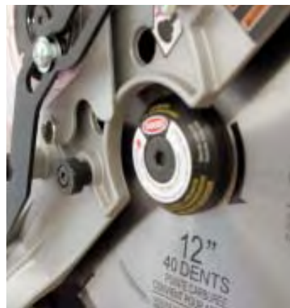
Figure 7. The rear-mounted laser on both Hitachi saws is bright, accurate, and powered by its own switch (left). Arbor-mounted lasers, such as this one on the Ridgid model (right), operate only when the blade is spinning.
