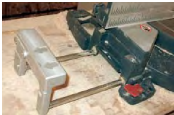
Figure 4. The Bosch 4212L includes the most useful auxiliary table extension as standard equipment (right). With Ridgid's 3½-inch table height, any scrap 2x4 can serve as a makeshift work support (below).
