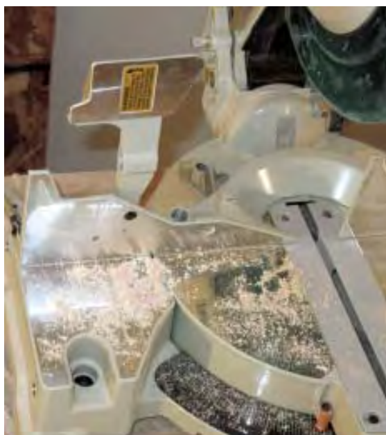
Figure 3. To make room for bevel cuts, models from Makita (left) and Hitachi (below left) are equipped with auxiliary fences that instantly flip out of the way; other makers' fences must be unfastened and slid away from the blade. Although convenient, two of the three flip fences tested were improperly aligned. The left fence on the Hitachi C12LDH was out of square by a full \frac{3}{16} inch (below).
