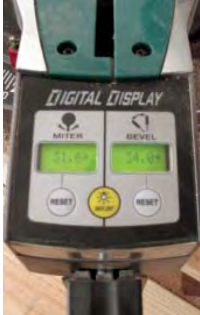
Figure 2. The Hitachi C12LDH's digital display made it easy to adjust angle settings, especially when cutting bevels.
