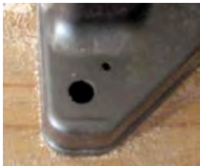
Figure 8. The Hitachi saws include two different-sized mounting holes in the base. Surprisingly, neither fits a standard drywall (or deck) screw without the use of washers or some other modification.
