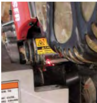
Figure 7. The rear-mounted laser on both Hitachi saws is bright, accurate, and powered by its own switch (left). Arbor-mounted lasers, such as this one on the Ridgid model (right), operate only when the blade is spinning.
