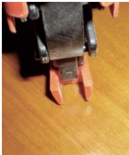
Figure 2. Most protective tips hamper visibility by making it hard to see where nails will enter the stock. Paslode avoids this problem by equipping its guns with a U-shaped tip (left). Bostitch supplements its gun's conventional tip with a package of profile tips (above) that can be used to index the nose of the tool to a variety of moldings.
