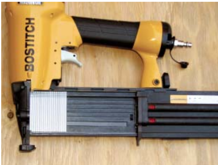
Figure 3. A side-opening magazine makes loading and unloading the Bostitch easy; it also provides access for clearing jammed fasteners.
