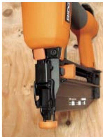
Figure 4. With most guns, clearing jams involves flipping open a luggage-style latch on the nose of the tool (above). Paslode created a sleeker, less cluttered nosepiece by building its latch into a contoured cover (above right) that blends smoothly into the casing (right).
