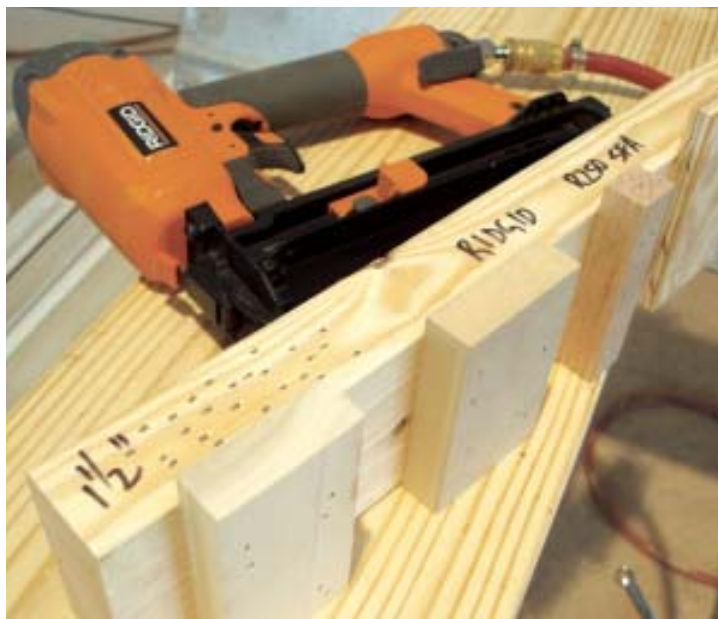
Figure 1. The author used this setup to test each gun's ability to set nails. First, he rapid-fired fasteners into the edge of a 2x4. Then, working at normal speed, he nailed on pieces of \frac{3}{4} -inch poplar, MDF, and oak. Many tools were unable to set all the nails.
