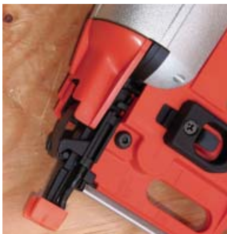
Figure 4. With most guns, clearing jams involves flipping open a luggage-style latch on the nose of the tool (above). Paslode created a sleeker, less cluttered nosepiece by building its latch into a contoured cover (above right) that blends smoothly into the casing (right).
