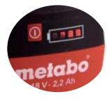
Because lithium-ion batteries run strong up until the end, some makers — including Milwaukee (left), Metabo (center), and Ridgid (right) — provide LED charge indicators to warn users they might not have enough juice to finish the job.
