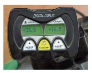
In addition to the usual scales, this saw has a digital display that indicates miter and bevel settings down to the nearest .5 degree.
