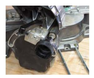
A knob connected to a rack-andpinion mechanism makes it easier to make fine adjustments to bevel settings. A similar micro-adjustment mechanism on the front of the saw controls miter settings. digital display: To make fine adjustments, you turn the knob and watch the display. I do have one gripe, however, which is that the knob for adjusting the miter would be easier to use if it were larger.
