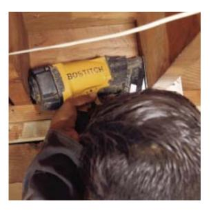
We tested the MCN150 by cycling it from van to van for several months so that each carpenter in the company could get a chance to use it. Our nail guns take a real beating, and we didn't go easy on this one. We dragged it through dirt and cobwebs in many different crawlspaces and used it to drive a lot of nails - usually into old, dry wood that was very hard.
