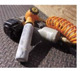
Shooting small fasteners rapidly or using a framing, siding, or roofing nailer can cause the tool's aluminum tank to frost, slowing air delivery.
