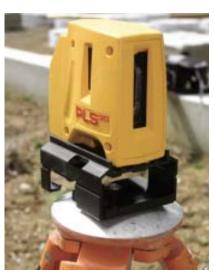
The user aligns the beam that projects from the bottom of the unit over the corner of the 90-degree angle he's laying out (left). When the PLS90E is attached to a surveyor's tripod, the down beam has a clear shot to the ground through the hollow fastening nut in the top of the tripod (right).
