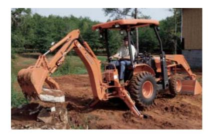
Multiple Attachments. While a loader/backhoe is already one of the most versatile pieces of heavy equipment you can buy, a three-point hitch increases its utility even further. The diesel-powered 26-hp, four-wheel-drive B26 TLB from Kubota has a 1,300-pound-capacity loader and a backhoe that can dig to nearly 8½ feet. A conventional three-point hitch accommodates such varied attachments as box graders, chipper-shredders, mowers, and snow blowers. Prices
