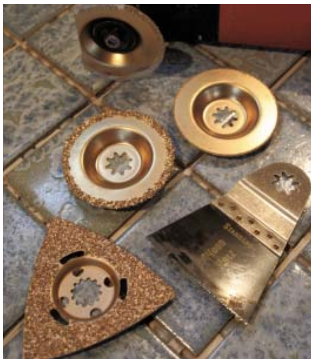
These tile accessories — a jamb-cutting blade, a triangular rasp, and three abrasive grout-cutting blades — have Fein's new star-shaped mounting holes.
